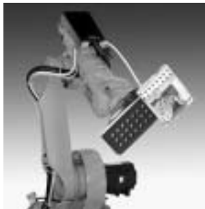
Application example: Safe handling, even with only part of the gripper active
